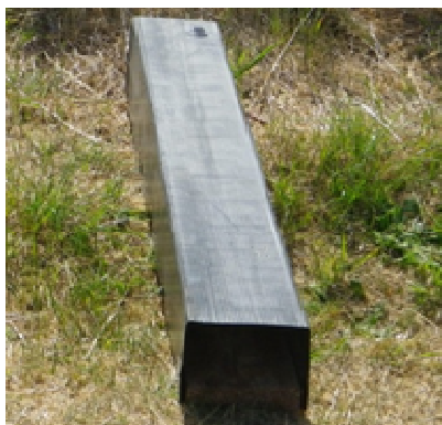
Plate 5 Shows a tracking tunnel. A plastic tray was placed inside the tracking tunnel with an ink pad in the center and two pieces of card at each ends.
